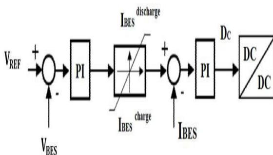
The  $I_{BES}$  is a current reference of the BES for controlling the transferred power through EV using a PI controller. The  $I_{BES}$  is restricted in capacity to the releasing rate 5C. The PI controls the duty cycle of the thyristors used in BES DC/DC converter within the set parameters. The power transfer to the vehicle is stopped when, the SOC<sub>BES</sub> arrives at 25%. The
