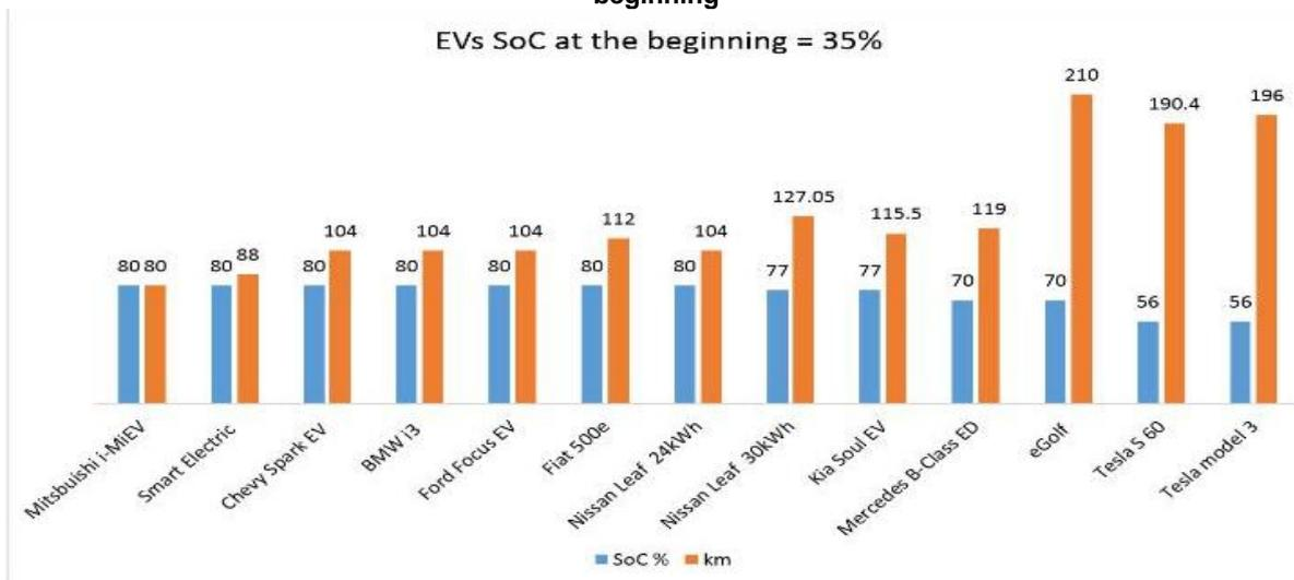
Figure 10 represents the chargeable limit of the DCFCS and the recharge capability of the EVs up to 80% SoC as per the EV<sub>SoC</sub> and the battery pack. The characteristics are plotted when EVs SoC are at 25% and 35%
