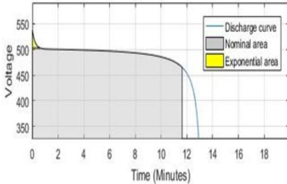
**Figure 3. SoC level determination through the V<sub>BES</sub>**
