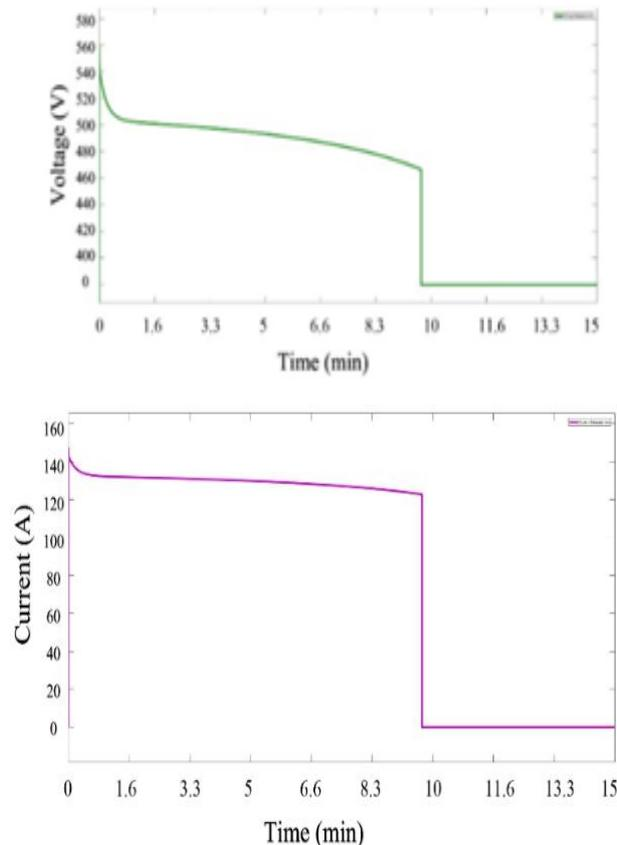
Figure 5 (a) produces diminishing characteristics of the  $SoC_{BES1}$ , the voltage drops in Figure 5 (b), and the steady current is 135 A. Figure 6 shows the EV's active power intake.
